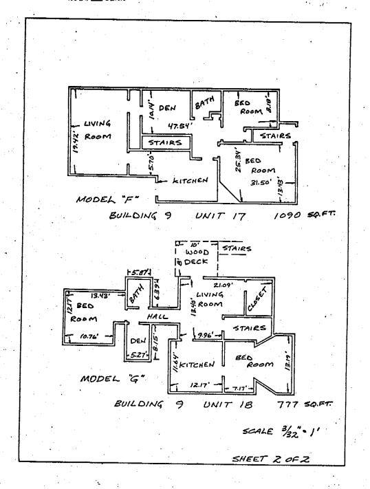
DISTANCES ARE MEASURED TO THE INSIDE FACE OF STUDS AT RANDOM LOCATIONS. NO CONSIDERATION HAS BEEN MADE FOR DIMENSIONAL VARIANCES CONTRACTED DURING CONSTRUCTION OR FOR MATERIAL NONCONFORMITIES. MEASUREMENTS ± 0.05'
